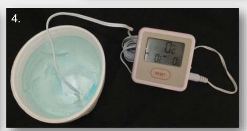
The thermometer must be accurate to ±1°C or better. If the temperature reading is more than 1°C above or below 0°C at 2 minutes, replace the battery (and record the date the battery was changed) and test again. If the temperature reading is still not within range, replace the thermometer.
